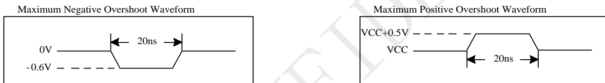
Figure 5-1 Maximum Overshoot Waveform
